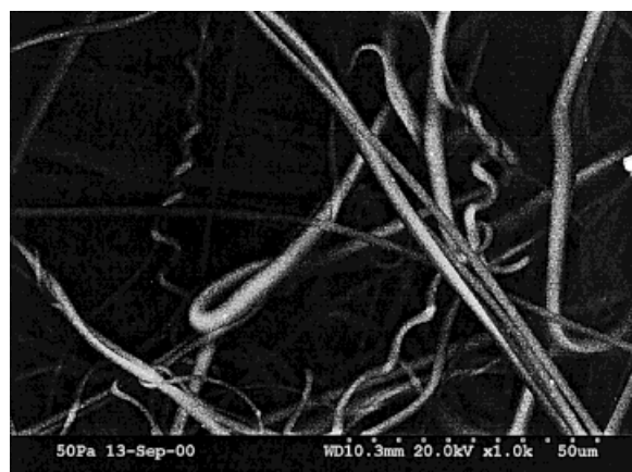
Figure 5 Curly Filaments in 50PTT/50PP Bico Meltblown Web.
